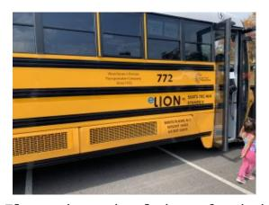
Electric school bus funded by Con Ed that is part of a test of vehicle-to-grid charging protocols.
