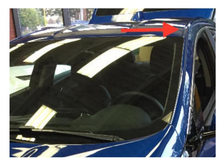
The aerodynamics of the vehicle have been further refined in the new model. There are strategically placed nips and tucks in the bodywork, including where the arrow is pointing in the photo. A small ridge has been molded along the side of the roof so the air is channeled over the back of the car rather than washed over the side.
