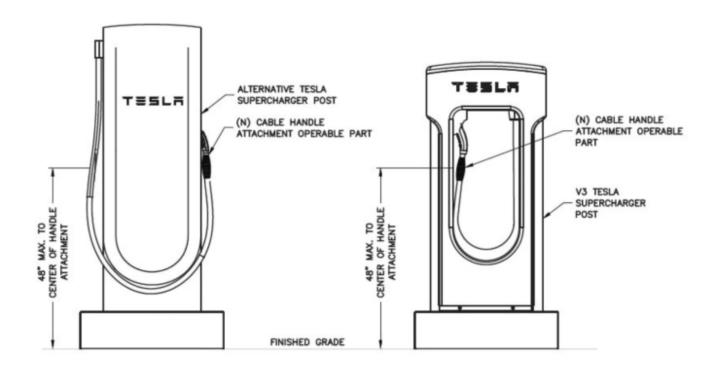
The V3 is on the right and the new V4 is on the left. Note the different style of connector with a considerably longer cord, external mounting, and much taller unit in general. That seems to be a good answer. Now we await word on the timing of the planned rollout, which may well be contingent on the timing of the grant funds.
