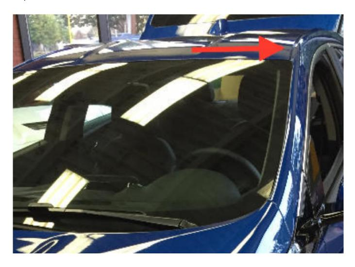
The aerodynamics of the vehicle have been further refined in the new model. There are strategically placed nips and tucks in the bodywork, including where the arrow is pointing in the photo. A small ridge has been molded along the side of the roof so the air is channeled over the back of the car rather than washed over the side. The center stack has been considerably reworked as seen in the photo below.
